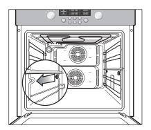
4. Remove the screw from the back by turning it anti-clockwise.
